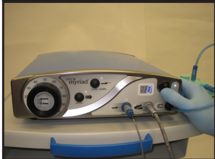
Figure 15: Console Power Up
