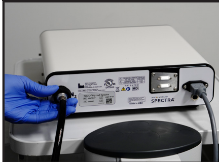
Figure 4: Nitrogen/Instrument Air Line Connection
