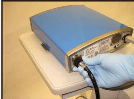
Figure 3: Nitrogen/Instrument Air Line Connection
