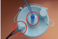
Check console aspiration line. Make sure both lines are plugged into canister.                        |
