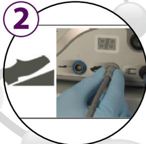
Plug in foot pedal connection to console.
